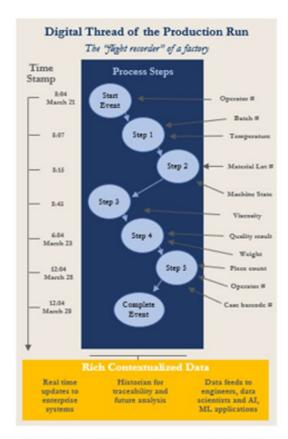
Digital thread captures all runtime meta data and contextualizes and transforms raw data into complex data model and useful information in real time.
