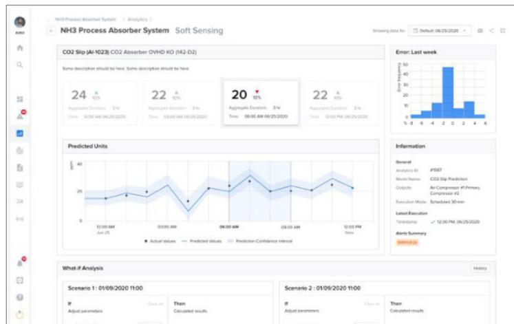
Forecasting process parameters using AI. These forecasts are fed back into the AI optimization models that can generate optimal control trajectories that optimize multiple objectives.
