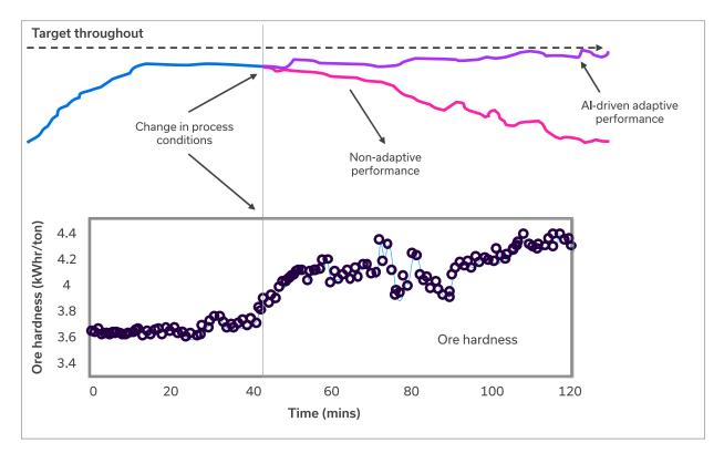
As ore hardness increases, Al-driven adaptive performance optimization helps maintain throughput levels without compromising grind quality.
